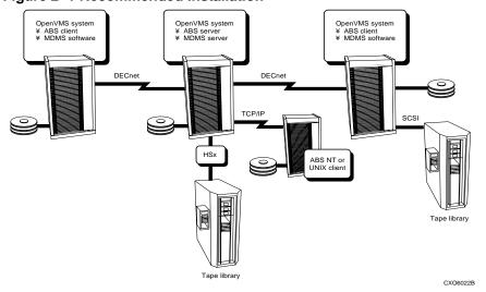
Figure 2-1 Recommended Installation
